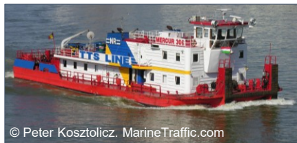
Type 1 pusher: 2 x 1194 kW/1800 rpm
