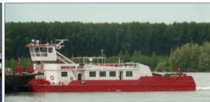
Type 3 pusher: 2 x 1185 kW/1000rpm
