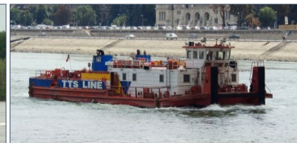
Type 4 pusher: 2 x 925 kW/750rpm
